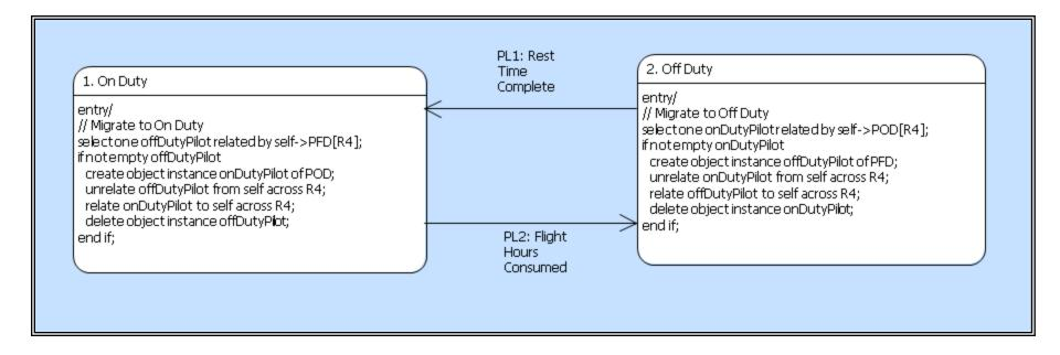
This is the state model for Pilot (PL). Note the creation of a new subtype to reflect the change of state (and the destruction of the old subtype). This technique is known as 'Type Migration'.
